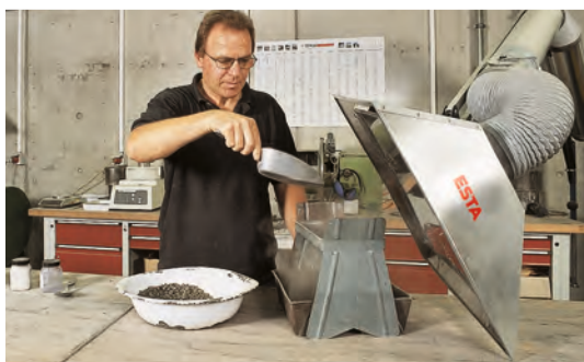
Extraction arm with square hood for large-scale extraction of dust in a transfer process in the bulk materials industry
