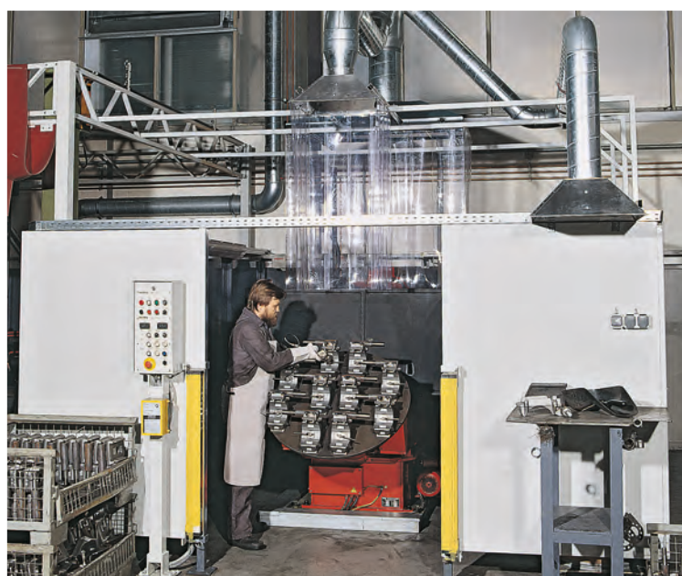
Square extraction hood on a welding robot
