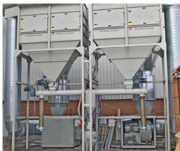
Central extraction system with two rotary valves for the continuous discharge of brick dust
