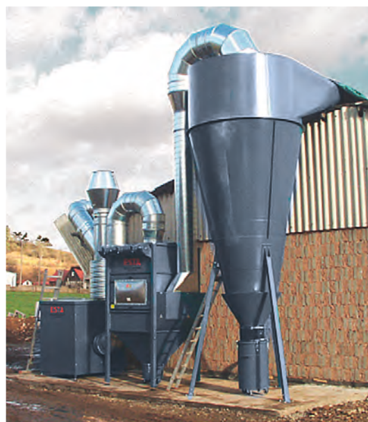
ESTA DUSTMAC F-144 with cyclone pre-separator for the extraction of zinc and cotton fibres with polishing wax
