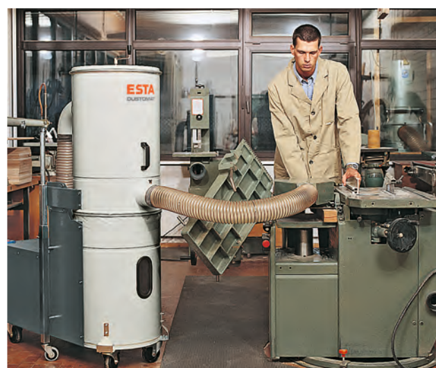
ESTA DUSTOMAT-10 with PU hose installed on a buzz saw for extraction of wood dust
