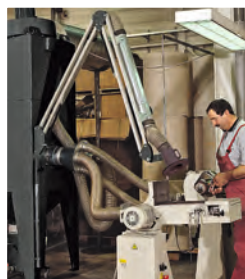
Extraction arm with oval hood for a grinding application
