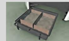
After the filtration process, the separated dust particles fall into a mobile 160 litre drawer below the filter chamber. Two collecting boxes inside are sealed with a lid before removal, which ensures low-dust disposal of the extracted material.\* A new, additional collection container collects coarse particles and sparks to protect the main filter and minimise the risk of filter fires.
