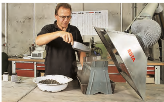
Extraction arm with square hood for large-scale extraction of dust in a transfer process in the bulk materials industry
