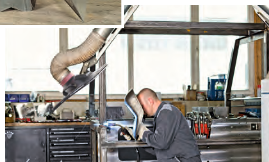
Extraction arms with efficiency hood for precise detection of welding fumes
