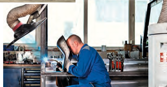
Extraction arms with efficiency hood for precise detection of welding fumes
