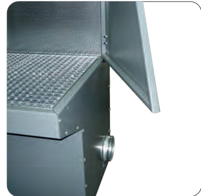
Side panel swung back for larger work pieces
