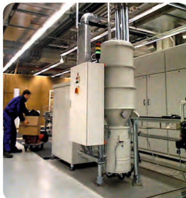
Cyclonic filter FZ-1003 with 100 Litre collection container
