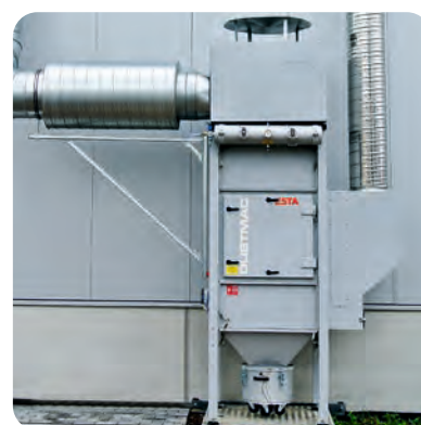
DUSTMAC F-144 in the metalworking industry
