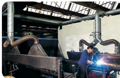
Slotted extraction hoods in the automotive industry
