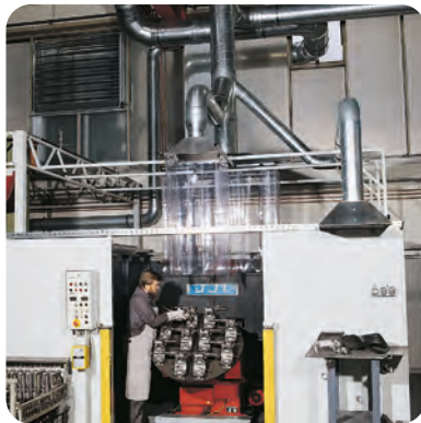
Extraction at a robotic welding station
