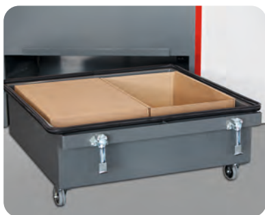
The detachable dust collection drawer with lockable cartons ensures simple, dust-free disposal.
