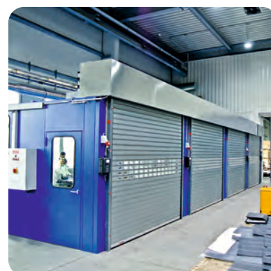
4-fold grinding cabin with rolling doors
