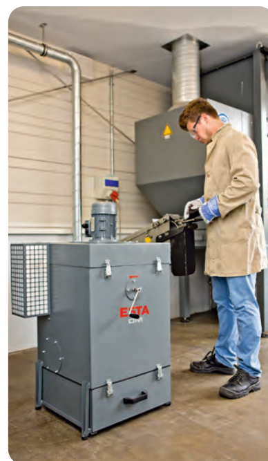
OM-8 connected to a belt sanding machine
