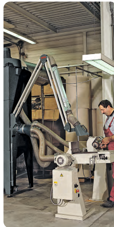
NA-K connected to a belt sanding machine
