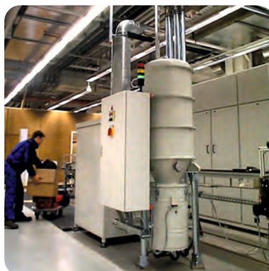
Cyclonic filter FZ-1003 with 100 Litre collection container
