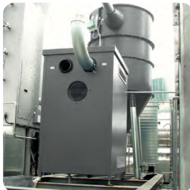
Filtration unit with explosion protection
