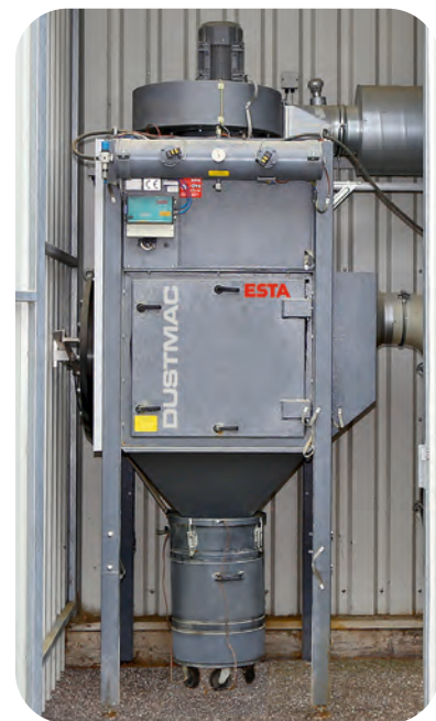
Central welding fume extraction system DUSTMAC F in the chemical industry
